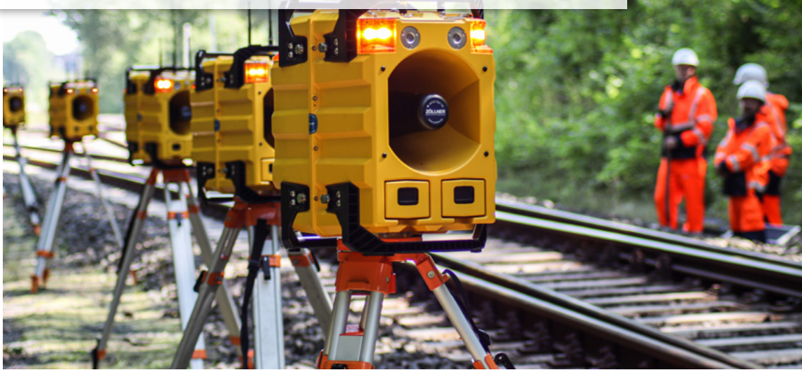
The automatic light and sound warning system warns of an approaching train
