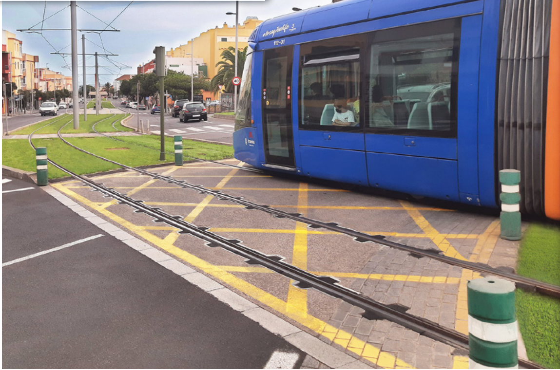
The tram in Tenerife runs on rails in the removable insulation chamber
